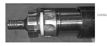
Alternatively, a 3/4 in. (19.05 mm) threaded rod with an appropriately sized washer and nut can be inserted into the guide and a female lifting eye can be attached to the opposite end. The casing can be hoisted vertically and the internal stack of parts can be lifted from the casing.
