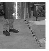
The QL120 ships with a lifting plug which threads into the air distributor.
