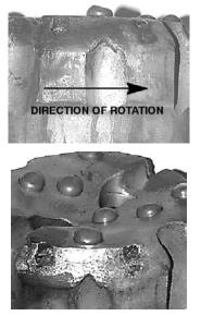
View showing wear flat on leading edge - indicates rotation too slow. note that carbide failure was caused by the leading edge wear flat.
