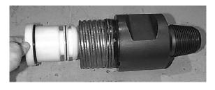
3. There is no need to remove **the inducer** unless damage is visible. **(Only inducers with snap rings can be removed).**
