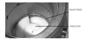
4. If the **inducer** has to be removed, press out the old one and press in the new one.
