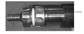
The QL200 casing is not reversible so the cylinder stop rings halves must be reinstalled in the same direction they were removed.
