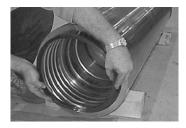
9. Insure the o-ring on the bearing is in good shape as it holds the bearing in place when the chuck is removed. Slide the bearing into the casing until it seats against the bearing stop ring. The bearing may need to be tapped from side to side to prevent it from getting stuck in the bore.
