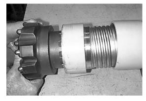
This can be accomplished with all of the DTH 's laying horizontal, except for the QL200. It may be preferable to hang the QL200 vertically from a hoist, use a wrench and break lose the joint, and spin the casing while slowly lifting the DTH.
