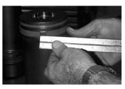
It is useful to pre-stress the seals slightly so they don't get caught in casing grooves when installing piston.
