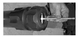
■ Measure the piston large diameter in the location shown.
