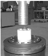
On the QL200, install the belleville springs and spacer.
