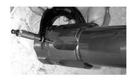
12a Non-lube piston, seals and bearing inspection (Replacement seals and bearings are available as a kit only)
