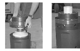
2. If the casing needs to be reversed, slide the cylinder, distributor and valve cap assembly into what was the chuck end. Otherwise slide the assembly into the backhead end. Note that even though the casing may not require reversal due to OD wear, it may be worthwhile to reverse the casing to renew the end of the bore the piston slides in. On the QL50/QL55QM, QL60/QL65QM and QL80 the cylinder stop ring in the casing does not need to be moved.
