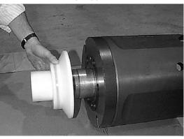
10. Moving back to the chuck end, pull the bit bearing from the hammer casing. Depending on the degree of rust or dryness of this area, a bearing puller may be needed to remove the bearing. When using a puller, be careful not to catch the bearing retaining ring. Sometimes lifting and dropping the casing on a block of hardwood can jar the bearing loose.
