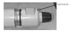
Torque all backheads until the backhead to casing gap is closed. This will require roughly 1500 ft-lb per inch (.86 kN-m per mm) of hammer for the QL50/QL55QM, QL60/ QL65QM and QL80. For example, the QL80 is an 8 in.
