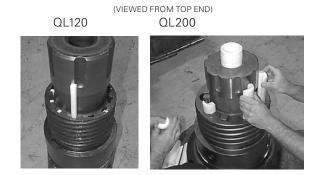
11. Install the bit retaining rings and bit retaining ring o-ring on to the bit and chuck.
